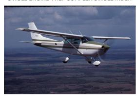
The **Cessna 182 Skylane** is an American four-seat, single-engined light airplane, built by Cessna of Wichita, Kansas. It has the option of adding two child seats installed in the baggage area.
